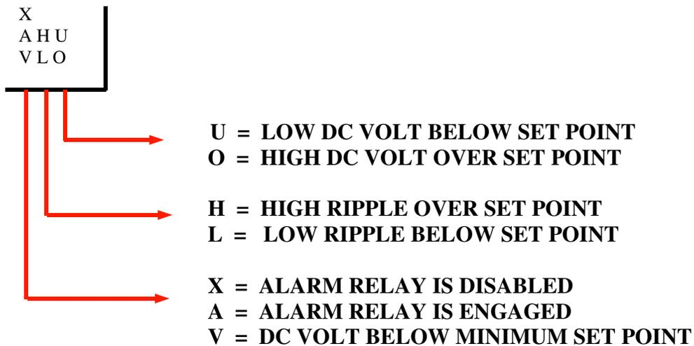
**The enabled ALARM engages when one or more of the set points are out of range. The ALARM disengages when all set points are within their ranges.**
